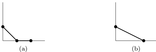
FIGURE 1. (a) One segment of the Newton polygon of f has x -length 1 and slope -1 , while the other has x -length 1 and slope 0. (b) The Newton polygon of f has a single segment of x -length 2 and slope -\frac{1}{2} .
