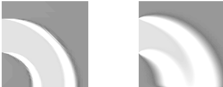
FIGURE 2. Comparison of the boundary layer behavior at the outflow boundary for the full upwind flux (left), and the Lax-Friedrichs flux (right).
