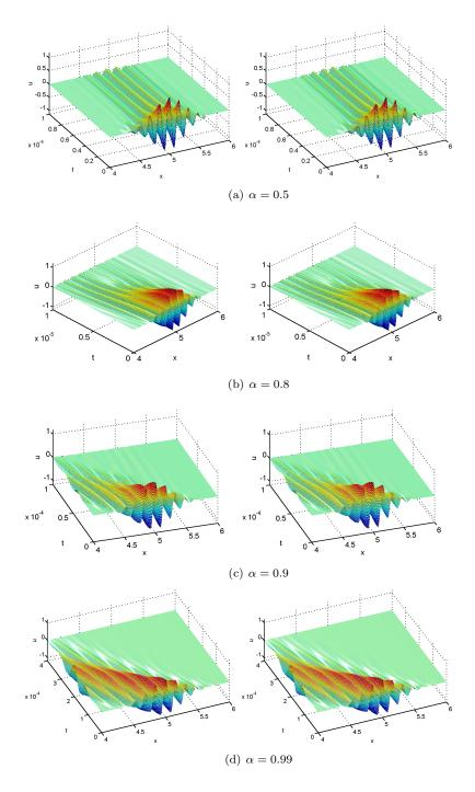
FIGURE 5. Example 3: The evolution of the reference solution (left) and the numerical solution (right). In this calculation,  $x_l = -6$ ,  $x_r = 6$ ,  $h = 10^{-3}$ , N = 1000.  $T = 1 \times 10^{-8}$  for  $\alpha = 0.5$ ,  $T = 1 \times 10^{-5}$  for  $\alpha = 0.8$ ,  $T = 1 \times 10^{-4}$  for  $\alpha = 0.9$ ,  $T = 4 \times 10^{-4}$  for  $\alpha = 0.99$ .  $\Delta t = T/N$ .
