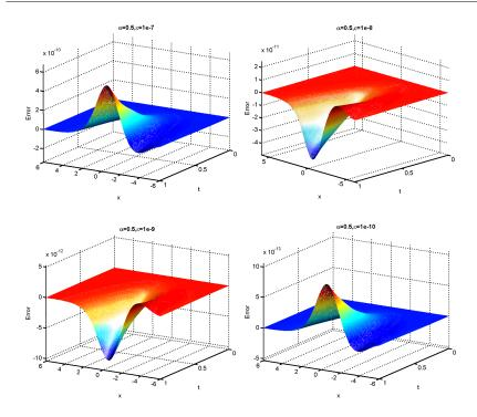
FIGURE 1. Example 1: The evolution of the difference (i.e., Error =  ${}^{F}U_{h}^{n} - {}^{D}U_{h}^{n}$ ) in the solutions to the direct scheme (4.21)– (4.24) (denote by  ${}^{D}U_{h}^{n}$ ) and to the fast scheme (4.50)–(4.53) (denote by  ${}^{F}U_{h}^{n}$ ) for  $\varepsilon$  = 1e-7, 1e-8, 1e-9, 1e-10, respectively. In the calculation, we set M = 120, N = 1000, and  $\alpha = 0.5$ .
