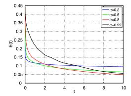
FIGURE 7. Example 3: The evolution of the energy of the wave remained in the bounded computational domain for different values of  $\alpha$ . In this calculation, we take M = 1000, N = 1000,  $x_l = 0$ ,  $x_r = 10$  and  $T = 4 \times 10^{-4}$ .
