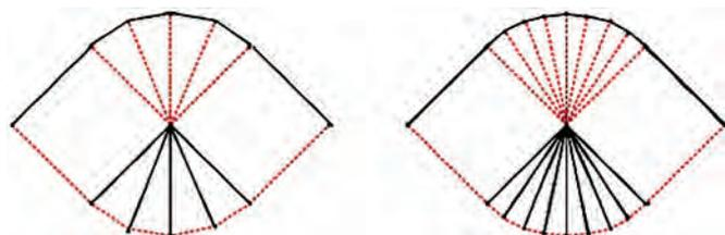
Figure 2. The frames  $[\lambda^n, \mathcal{A}^n]$  when  $n = 13$  and  $n = 21$ , where dotted red lines are in tension and thick black lines are in compression.
