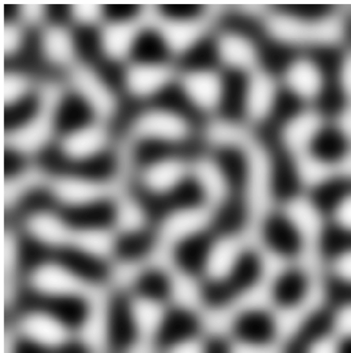
FIGURE 1. The geometry of a typical pattern observed during spinodal decomposition in the Cahn-Hilliard equation, where \Omega = (0, 1)^2 and \varepsilon = 0.015 .
