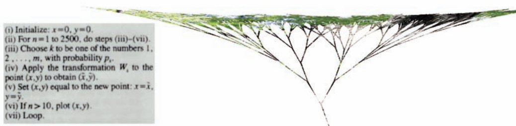
Figure 4. The original pseudocode from Byte magazine (January 1988) for implementing the chaos game algorithm to obtain an image of the attractor of an IFS on \mathbb{R}^2 . Notice the small number of iterations used! Nowadays, usually, I use 10^7 iterations and discard the first thousand points. On the right is a sketch of a 2-variable tree obtained by a generalization of the chaos game.
