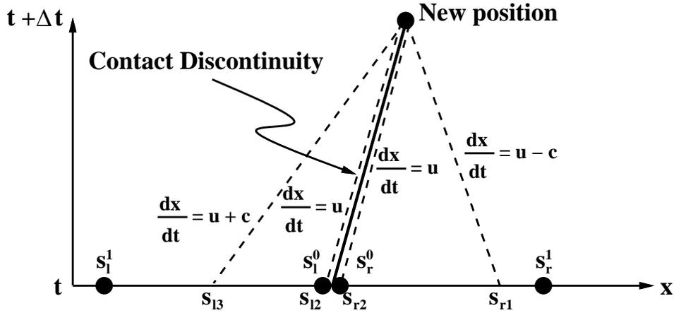
FIGURE 2. A schematic picture of the data used for the normal propagation of a contact discontinuity. The front data at the old time step provides a Riemann solution, that is corrected by interior data, using the method of characteristics.
