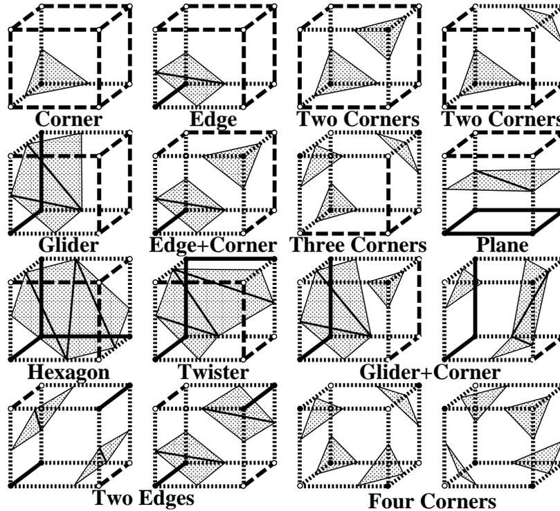
FIGURE 3. Grid based interface reconstruction. For a two-fluid interface within each grid cell, there are  $2^8 = 256$  possible configurations for the crossings of the cell edge by the interface. Through elementary operations of rotation, reflection, and separation, these cases can be reduced to the sixteen cases shown above.
