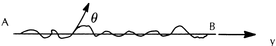
FIG. 4. Newly formed grain boundary after welding
