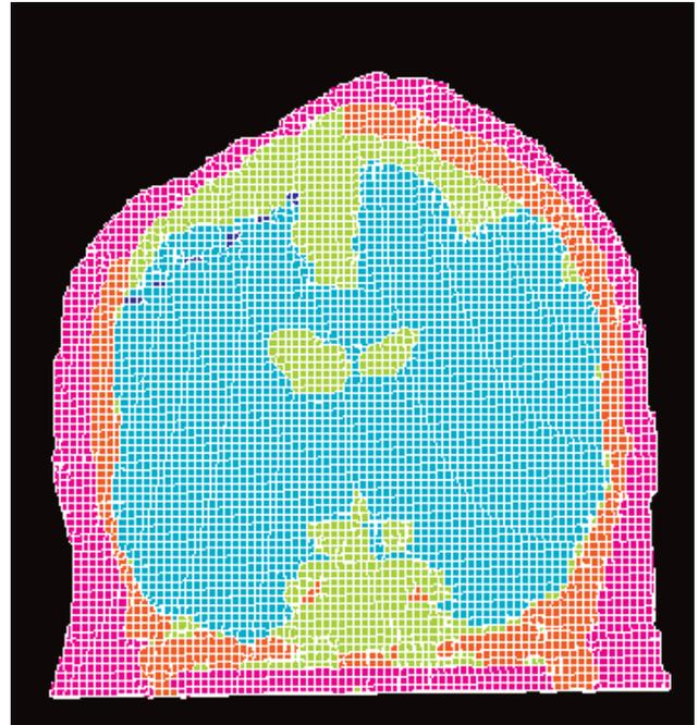
**Figure 1.** 2-mm geometry-adapted finite element hexahedral mesh of a segmented computer tomography and magnetic resonance data set for a patient with medically intractable epilepsy. The tissue layers—skin, skull (with the surgical opening visible), cerebrospinal fluid, and brain—and the depth electrodes are shown in different colors.
