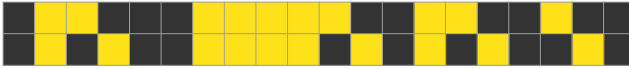
Figure 1.16. The top row represents a line of taxis (yellow coordinates) driving down a road (black coordinates) to the right ( \rightarrow ), and the second row represents the taxis one time unit later.
