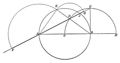
Draw the line AC cutting the arcs ODC and AB at D and J; also draw the line BDE through B and D cutting the given circle at E. Then  $AD + 3DE = \pi r$  approximately.
