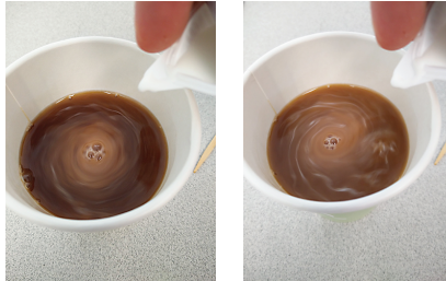
FIGURE 1. Milk mixing into an approximately axisymmetric vortex
