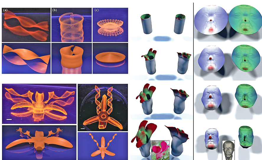
FIGURE 9. Examples of solutions of inverse problems in morphogenesis—to program the metric structure and thence create complex shapes from flat sheets. On the left are shown experiments with 3d printed gel structures that swell in a good solvent, along with representative numerical solutions that are based on minimizing the energy (4.1). (This figure is from [47] by Gladman, Matsumoto, Nuzzo, Mahadevan, and Lewis, Biomimetic 4D printing , Nature–Materials , 15 (2016), 413–418; © 2018, Springer Nature.) On the right [120] we see results of the solution of inverse problems to grow a flower from a bilayer cylindrical shell, and a face from a circular bilayer disk.
