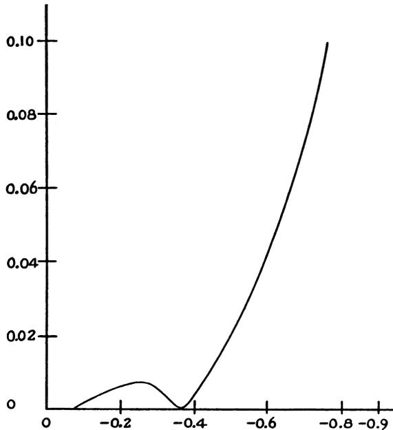
Convergence of  $u_2$ : The ordinate is the fractional difference between the second and first approximations  $[u_2^{(2)} - u_2^{(1)}]/u_2^{(2)}$  for the set of four simultaneous equations which describe one hypothetical free-radical flame. The maximum fractional error is always less than thirty percent and reaches 10 percent only after  $u_2$  has dropped to one thousandth its initial value. The convergence of  $u_1$  is equally good.
