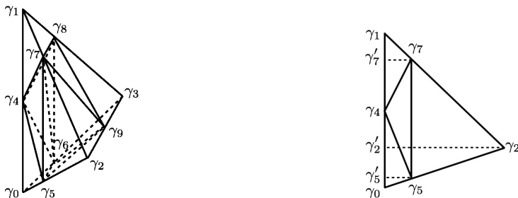
FIGURE 3. The mesh on an e -tetrahedron after one refinement (left); the induced triangles on a face containing the singular edge (right).
