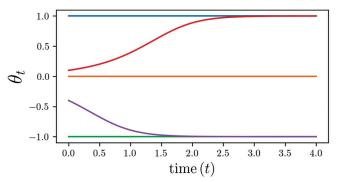
**Figure 1.** Five trajectories of the one-dimensional gradient system (2.2) with double well potential (2.6). The objective *V* has critical points at  $\theta = 0$  and  $\theta = \pm 1$ . The intervals  $(0, \infty)$  and  $(-\infty, 0)$  are basins of attraction for  $\theta = 1$  and  $\theta = -1$ , respectively.
