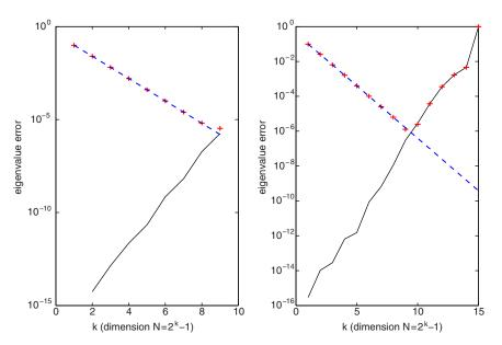
FIGURE 1. Example 1. Left: 2-D problem; Right: 1-D problem. solid line: computation error; dashed line: discretization error; +-line: overall error.
