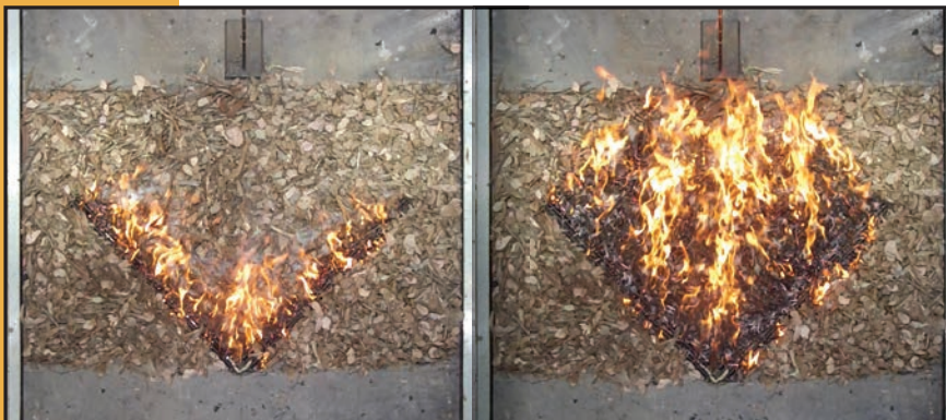
Wind tunnel fires meeting at an apex. Photo courtesy of Dr. Andrew L. Sullivan for Commonwealth Scientific and Industrial Research Organization.
