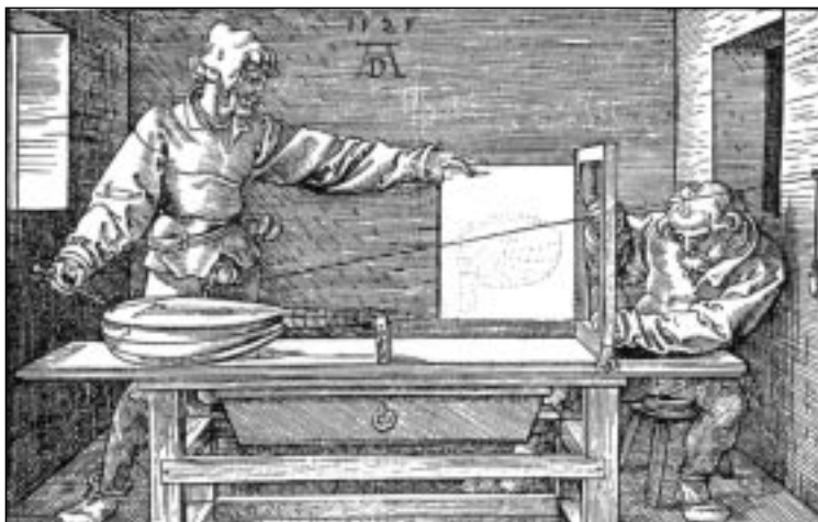
Albrecht Dürer woodcut, 1525, depicting an instrument being used to draw the perspective image of a lute.
