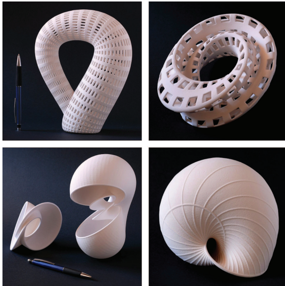
Figure 12. Photos of 3D printed models of three versions of the Klein bottle made by a Z-Printer Z310 Plus (material: plaster). Top left: Klein bottle according to parametrization (9)-(10); top right: Klein bottle according to parametrization (1); bottom left: Klein bottle cut in two parts, according to parametrization (2); bottom right: one half of the same surface, cut in such a way that each of the two halves is a Möbius band with circular border; some circular arcs lying on the surface itself are highlighted. (Models and pictures were created by the author.)
