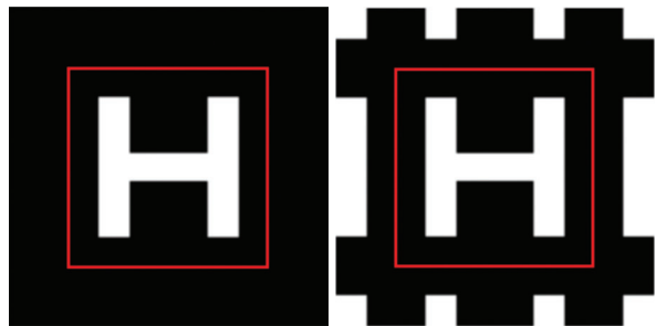
Figure 3. Image with assumed zero boundary conditions is shown on the left and one with assumed periodic boundary condition is shown on the right. The red box represents the FOV.
