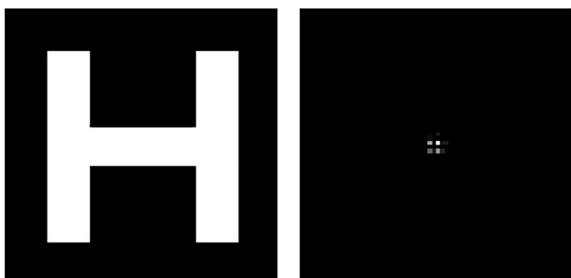
Figure 7. On the left we see the original image \mathbf{x}^{\text{true}} while the right shows \mathbf{x}^{LS} , the solution to the equation \mathbf{Ax} = \mathbf{b} , where \mathbf{b} is the noisy recorded image.
